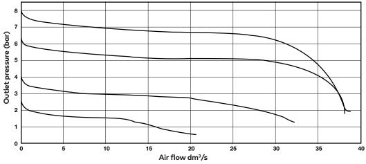
Inlet pressure: 10 bar (145 psi) Range: 0.3 to 10 bar (4 to 145 psi) Port size: 3/8", 40 µm element
